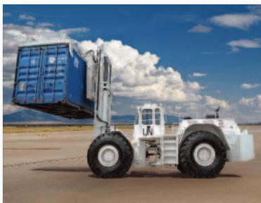
Built to military specifications with capacities up to 70,000lbs. Designs include; RT container handler, shipboard approved, air transportable, and custom configurations.
