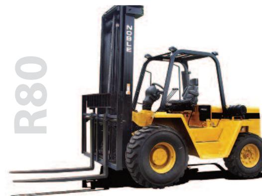
Noble "R" Series forklifts offer leaf spring suspension with ruggedness and capability that customers have been accustomed to for decades. The "RC60LP" Series offers compactness and easy maneuverability not normally associated with a true rough terrain forklift.
