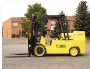
Cushion tire industrial workhorse with capacities from 18,000lbs to 40,000lbs. Propane or Diesel clean-burn engines with electronic transmission control.
